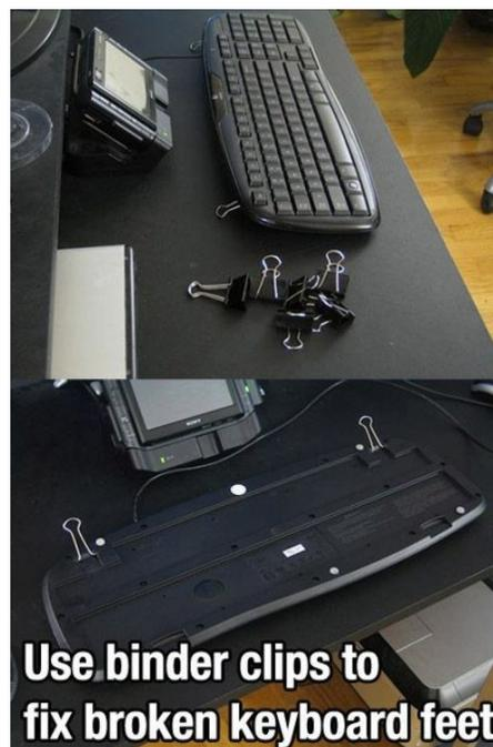
**Use binder clips to fix broken keyboard feet**
